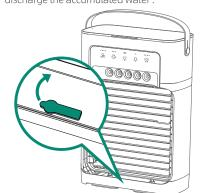
3 When not using the spray function, pour out the water in the water tank to prevent water leakage and bacteria grouwth.
