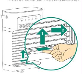
3 Make sure the power supply is disconnected, lift the middle part of the bottom of the fan grid and move it outward. Then clean it with a damp cloth or brush.
